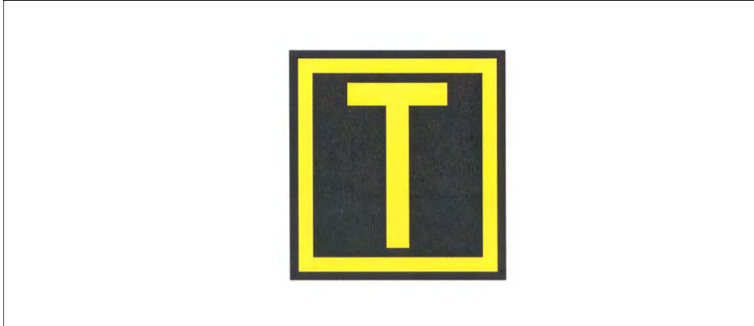
FIG 2-3-30 Taxiway Location Sign
