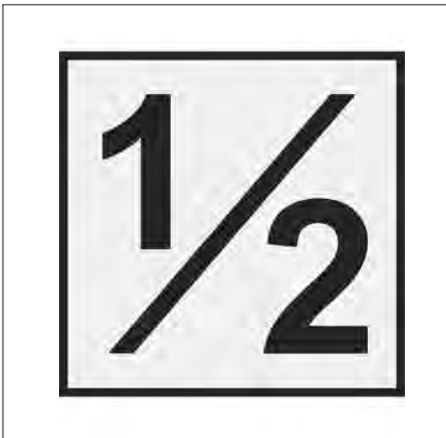
FIG 7-5-1 Typical Runway Half-way Sign
