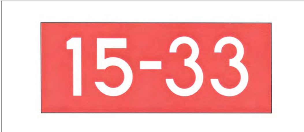
FIG 2-3-24 Runway Holding Position Sign
